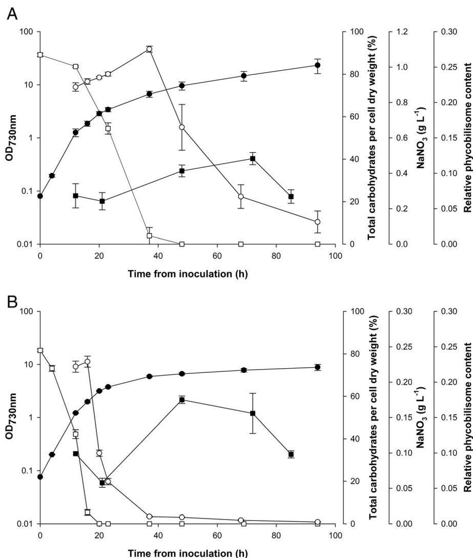
**Figure 1** Cultivation of *Synechococcus* with different nitrate concentrations. (A) Initial NaNO<sub>3</sub> concentration of 1 g L<sup>-1</sup>. (B) Initial NaNO<sub>3</sub> concentration of 0.24 g L<sup>-1</sup>. Solid circles: OD<sub>730</sub> (optical density at 730 nm); solid squares: total carbohydrates per cell dry weight (% weight per weight); open squares: NaNO<sub>3</sub> concentration (g L<sup>-1</sup>); open circles: relative phycobilisome content per cell. h, hours.
