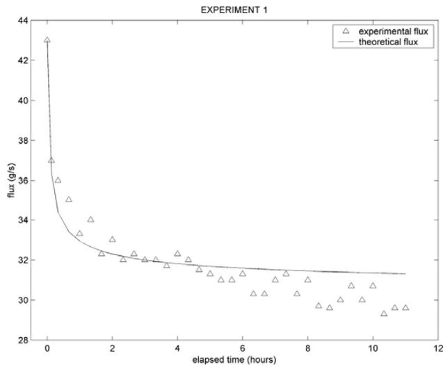
**Fig. 3.** Flux results (triangles) from experiment number one. An initial transient of about 3 to 4 h is visible, afterwards the flux reaches a steady state. Overimposed solid line represents the theoretical curve which best fits the experimental data.
