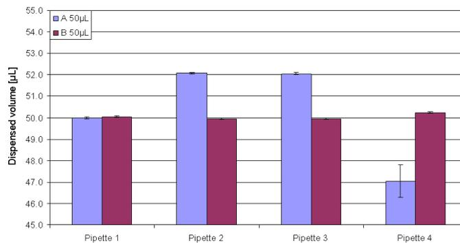
Figure 4: Two different volume verification runs both using 5.0 $\mu$ L as target volume on an eight channel fixed tip Sias Xantus robot. Run A showed unacceptable pipetting. Run B following calibration showed acceptable pipetting.
