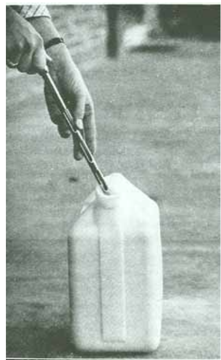
Figure 1. Sampling seed with a slotted trier.
