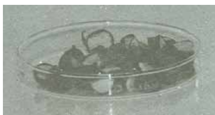
Figure 7: An acorn sample ready for drying in a microwave oven. Note that the dish is in the center of the oven floor.
