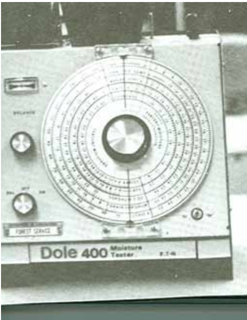
Figure 6. One type of electric seed moisture meter that can be used on some tree seeds
