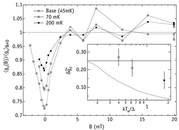
FIG. 3: (a) Normalized average peak height as a function of perpendicular magnetic field, for the  $0.7 \mu\text{m}^2$  dot at several temperatures. Inset shows  $\delta \tilde{g}_o$  for each temperature, along with theoretical curves from Ref. [11]. Note crossover from solid to dashed curve at  $T_e \sim 200 \text{ mK}$ .
