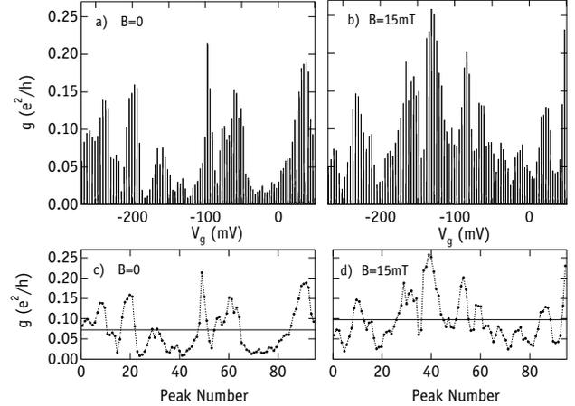
FIG. 1: Coulomb blockade peaks at electron temperature  $T_e = 45 \text{ mK}$ , for the  $0.7 \mu\text{m}^2$  device at (a)  $B = 0$  and (b)  $B = 15 \text{ mT}$ . Every second peak was measured, as peak-to-peak correlations made measuring each peak inefficient. (c,d) Peak heights, extracted from (a,b). Horizontal lines show average peak height, indicating suppression of average height at  $B = 0$ .
