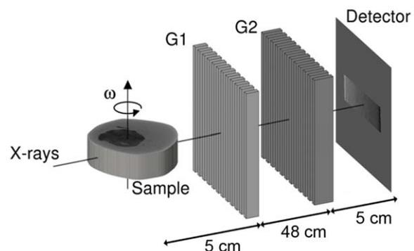
**Figure 1. Experimental setup.** Not to scale. The sample is placed in front of the interferometer as close as possible to the first grating. The distance between the two x-ray optical transmission gratings, G1 and G2 is dictated by the fractional Talbot order. The detector is placed immediately after G2. The phase-contrast images are collected for each rotation angle  $\omega$  by scanning G1, along the transverse direction in four steps.
