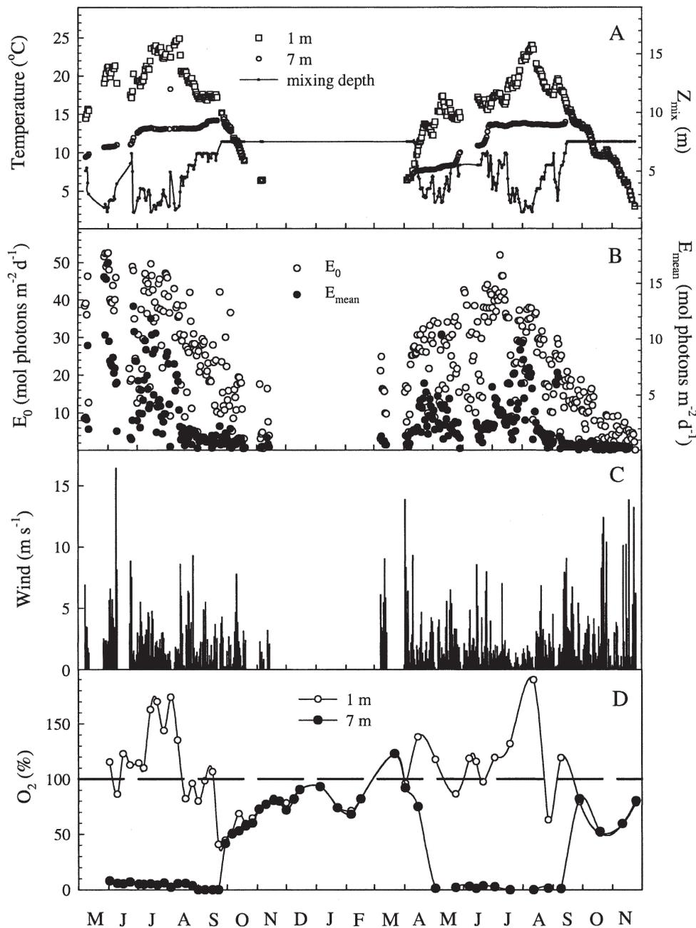
Fig. 3. Seasonal changes in daily water temperature, calculated mixing depth ( $Z_{\text{mix}}$ ), surface irradiance ( $E_0$ ), mean irradiance ( $E_{\text{mean}}$ ) in mixed surface layer, wind speed calculated at 10 m above lake surface, and weekly measurements of oxygen saturation in surface and bottom water.
