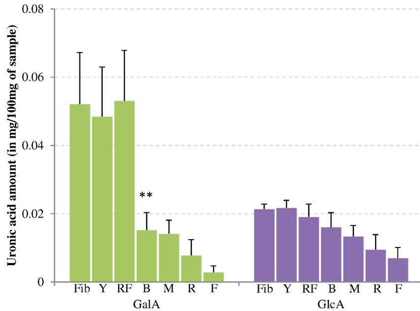
**Fig. 1. Uronic acid content of processed cotton samples.** Extracted galacturonic acid (GalA) and glucuronic acid (GlcA) from powdered textile processing samples; Fib = fibre, Y= yarn, RF= raw fabric, B= bleached/scoured fabric, M= mercerized fabric, R= ready-to-dye fabric, and F= finished fabric. Error bars represent standard deviation (n=3). \*\* indicates significant difference between bleached and raw fabric samples at  $p < 0.01$ .
