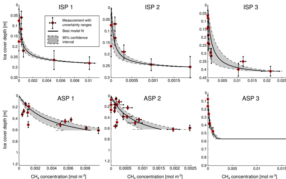
**Figure 6.** Measured and modeled  $\text{CH}_4$  concentrations with ice cover depth of different ponds. The whiskers show the measurement uncertainty and the shaded areas indicate the 95 % confidence interval of the model. The range of depth axis represents the maximum pond depth. Sampling was limited to a maximum ice cover depth of about 60 cm due to the length of the guide bar used with the chainsaw.
