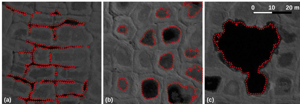
**Figure 2.** Typical ponds in the polygonal tundra mapped from near infrared (NIR) areal images. At the study site occur (a) ice-wedge ponds, (b) intra-polygonal ponds within intact polygonal structures, and (c) merged ponds show clear signs of degradation of the polygonal structures. According to their degree of degradation intra-polygonal ponds and ice-wedge ponds are classified as initial state ponds (ISPs) and merged ponds as advanced state ponds (ASPs).
