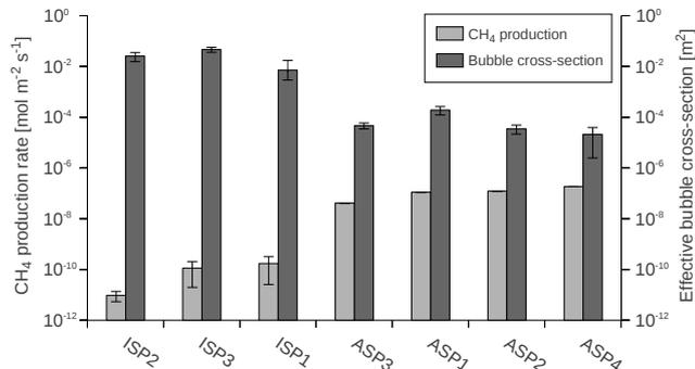
**Figure 7.** Net methane production and effective bubble cross-section for different ponds, calculated by inverse modeling using the 1-D mass balance model (note the logarithmic scale). The whiskers indicate the 95 % confidence interval of the model results.
