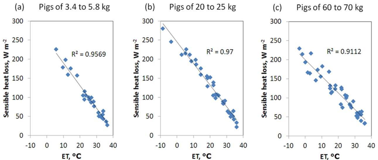
Figure 1. Sensible heat loss for pigs at different ET (Eq. 1) assuming  $c = -1.0$ ,  $d = 42\ ^\circ\text{C}$  and  $e=0.66$ . Data originates from Mount and Ingram (1965) and includes exposure to different ambient temperatures (15, 20, 25, 30 and 35 °C) at different air speed (close to 0.08, 0.35, 0.60 and 1.00 m/s). The three graphs represent different weight ranges.
