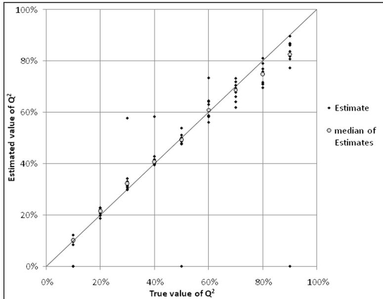
Figure 4: Monte Carlo Simulation results for nine values of  $Q^2$  with ten repetitions each. The MCEM-MLE estimates are compared to known true values. The circles indicate the median values of the estimates. Estimates lying on the  $45^\circ$  are exactly equal to the true value.
