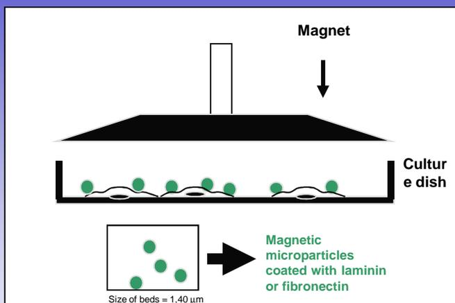
**Fig.1** A magnetic field of 0.5 mT was generated by an electromagnet (Power Generator 0-30 Volts, 0.1-100 Hz; Elcanic A/S, Denmark). The magnet produced alternating MF at frequency of 1 Hz. Magnet was placed 10 mm over the monolayer of cells during the stimulation period. Cells lacking beads but placed under the magnetic field were used as an additional control.
