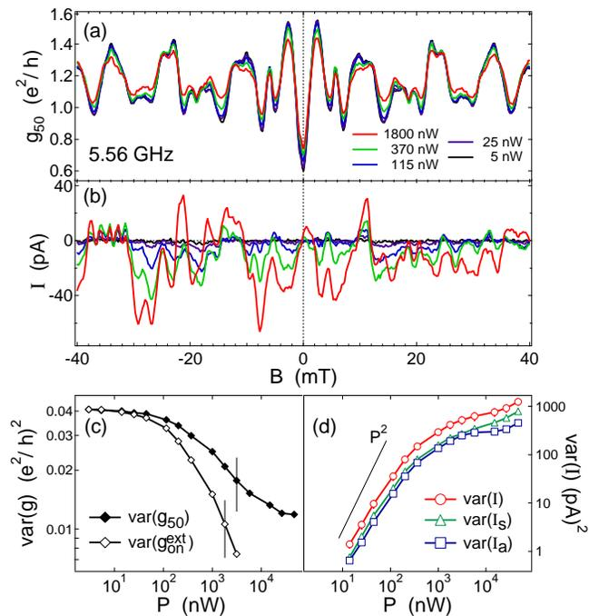
FIG. 3: Magnetic field dependence of (a) conductance and (b) rf-induced dc current, for increasing levels of incident power  $P$  at 5.56 GHz. Full sweeps spanned the  $-100$  mT to  $+100$  mT range. (c) Variance of the measured conductance  $g_{50}$  and of the extracted on conductance  $g_{on}$ , as a function of incident power. (d) Power dependence of the total induced dc current, and of its symmetric and antisymmetric components.
