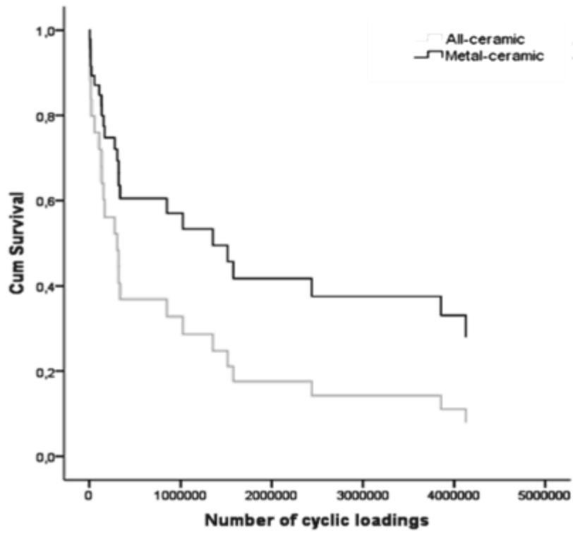
Figure 5. Estimated number of cyclic loadings until fracture of the veneering ceramics (fracture mode  $\geq 3a$ ); all-ceramic (AC, n=16) vs. metal-ceramic (MC, n=16) restorations
